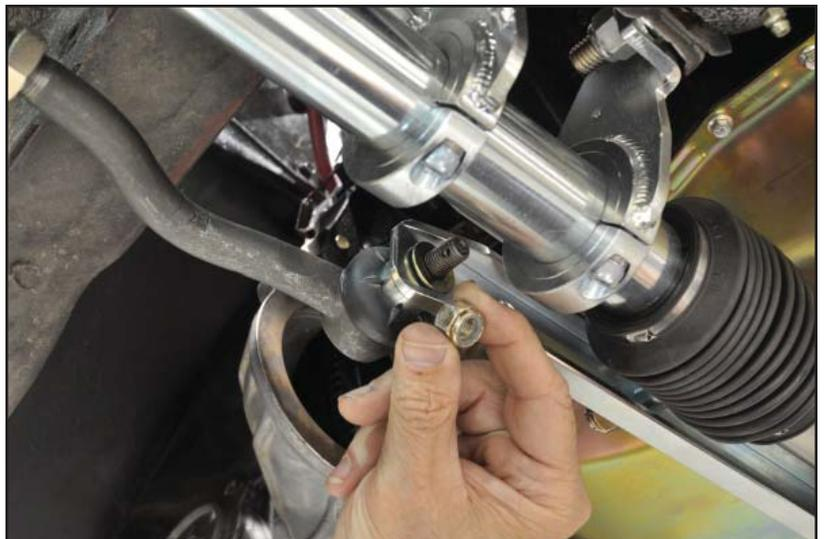
14. Tighten the locknut with a 3/4" wrench. You will have to push the tie rod into the tapered adapter while tightening the locknut.
