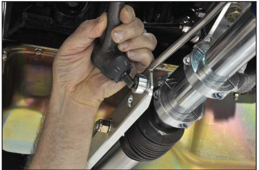
13. Place a 1/2" hardened flat washer over the tie rod stud, followed by a 1/2" locknut.
