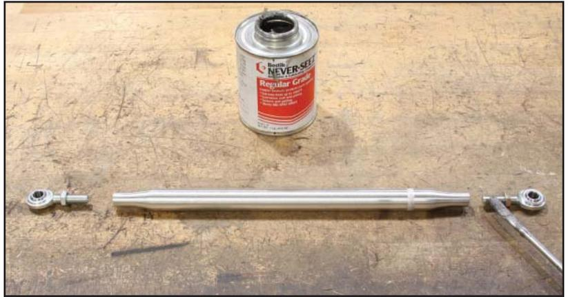
19. Bolt the radius rod assemblies to the firewall bracket using a 3/8-16 x 1-3/4" button head cap screw, tapered spacer (not shown) and locknut (2x). The rod end mounts below the bracket with the tapered spacer between the bracket and rod end. Narrow end of taper must be against rod end. Tighten to 30 lb-ft.
