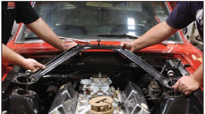
6. Bolt the firewall bracket to the firewall lip using the existing mounting holes. Secure with 3/8-16 x 1" button head cap screw, two flat washers and a locknut (4x). Bolts should only be snug to allow the bracket to shift with light force.
