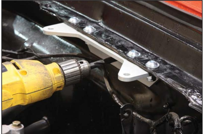
8. Secure with 3/8-16 x 1-1/4" button head cap screw, two flat washers and a locknut (3x). You will need someone on the other side of the firewall to help.
