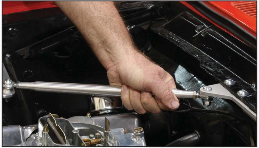
25. Tighten the jam nuts to 30 lb-ft.
