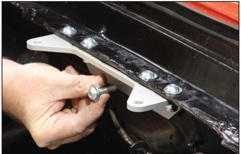
IMAGE: Insulation normally runs up to the top of the firewall and ends at the sheet metal seam. The insulation can be easily pulled down to install the support plate, flat washers, and locknuts.
