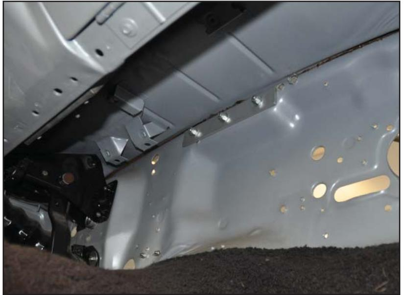
12. Place the aluminum shock tower plate over the shock and onto the OEM bolts.
