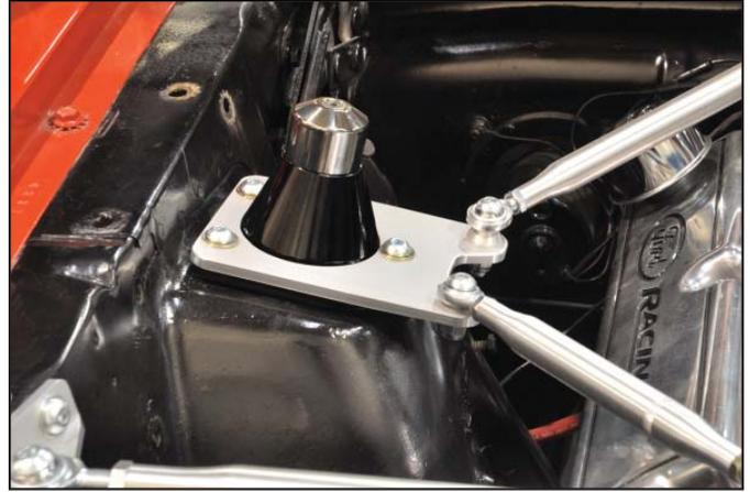
*Bolt-On Coil-Over mounted BELOW - standard ride height*
