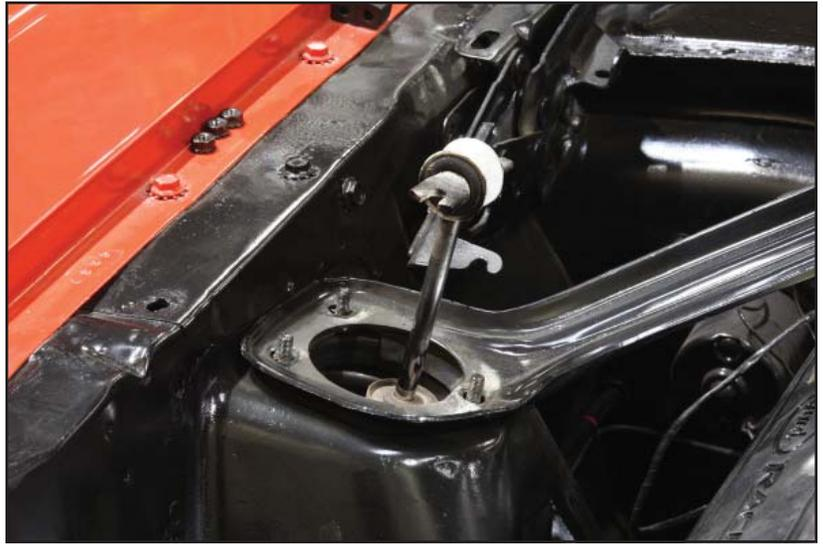
3. Unbolt the factory export brace from the firewall. Some OEM braces may be spot welded to the firewall lip. The spot welds will have to be ground or drilled out to remove the brace.
