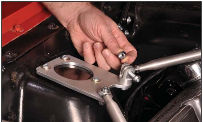
24. After both rod ends have been mounted, adjust the rod end so that it is not preloaded and can rotate freely.
