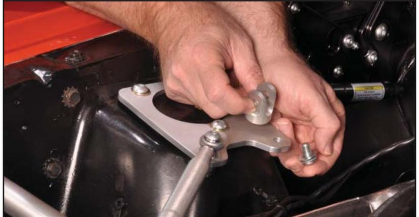
22. Install the 3/8-16 x 1-1/2" button head bolt and locknut (2x) to secure the radius rod at the shock tower end.
