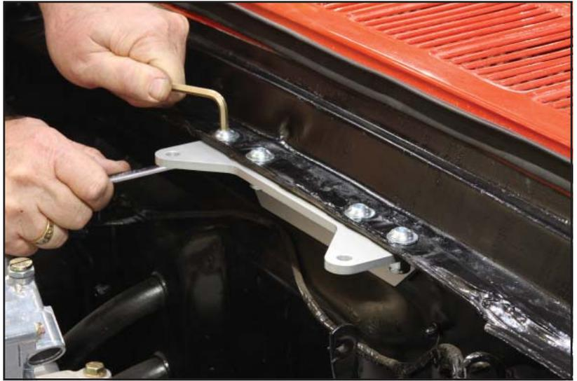
7. Using a 3/8" bit, drill through the firewall, using the aluminum bracket as a drill jig.
