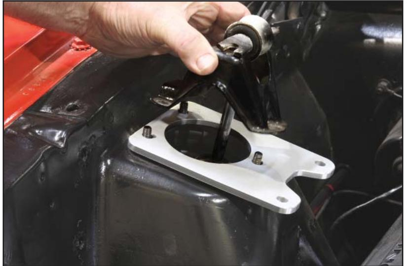
14. Use OEM hardware to secure the shock mount and shock crossbar.
