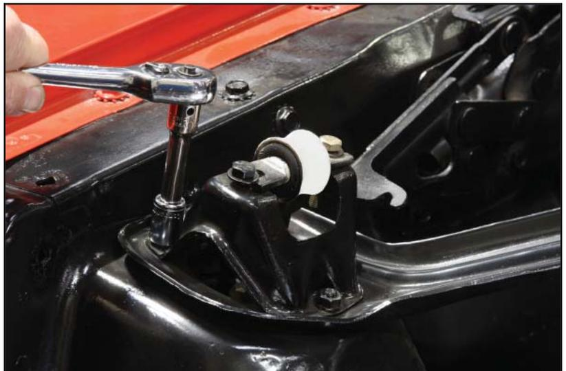
2. Remove the shock mount from the shock tower.
