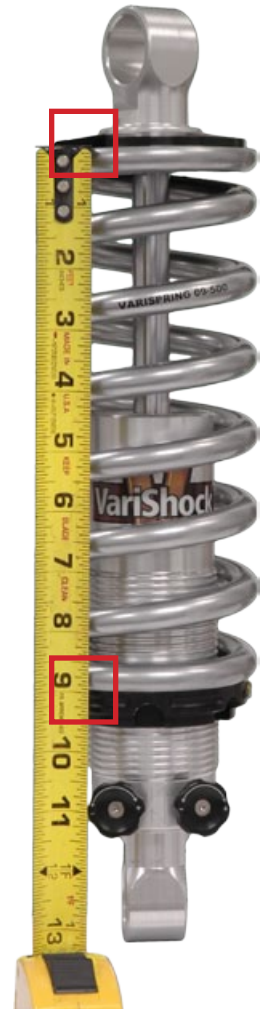
Measure the bottom end of the spring.
