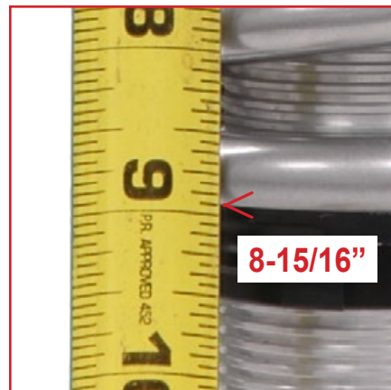
Measure the bottom end of the spring.
