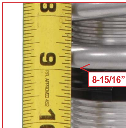
Measure the bottom end of the spring.
